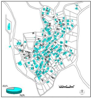
Figure 14: Thematic map showing the main axis of the buildings: parallel (cyan) and vertical (grey) to the slope.
