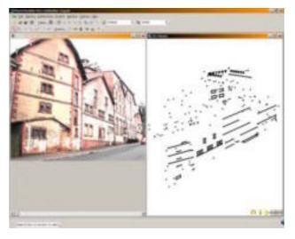
Figure 5. Malt house virtual model. The trace of slabs in the facade and some windows facing the street can be seen (PhotoModeler software).
