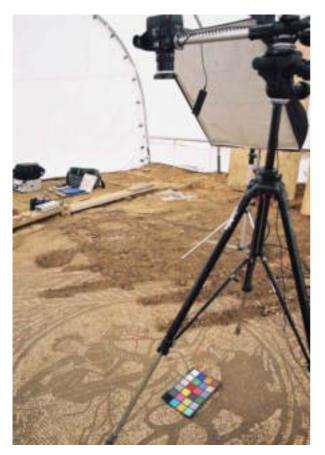
Figure 1 Rollei 6006 semi-metric camera set up on an extension bar with a Macbeth chart in the image.
