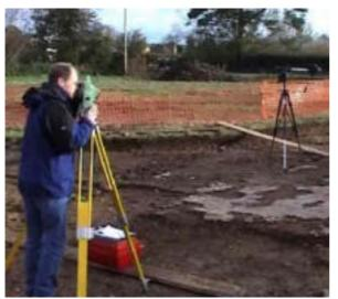
Figure 2 A Leica TCRM1103 is used to co-ordinate control targets
