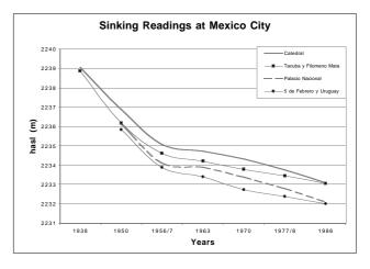
Figure 1. Table of readings of height above sea level through time in four points at downtown Mexico City
