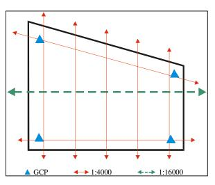
Figure 3. Sketch of the GCPs and flight strips.
