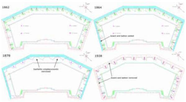
Fig. 5: Roof plans showing the different eras of the fort
