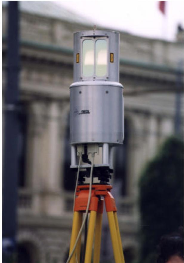
Figure 1 – LMS-Z210 laser-scanner
