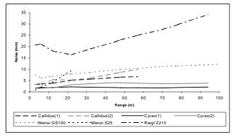
Fig. 9: Measuring noise in range direction (std. dev. for a single point) for different scanners on gray surface (40% reflectivity).
