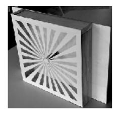
Fig. 6: Target with slots of varying widths for resolution tests.
