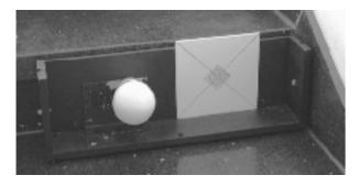
Fig. 1: Box for positioning spheres at defined locations on steps
