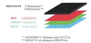
Figure 2. Structure of the solid image
