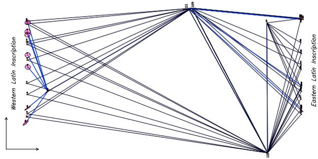
Figure 2 - Plan of the Control Network for the Latin inscriptions composed by five theodolite stations
