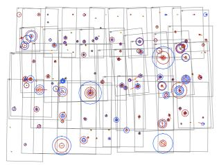
Figure 7 - Western side . Results of the aerial triangulation and photogrammetric models. Distribution of the control points, of the pass points, of the planimetric and altimetric observation residuals. The rectangular polygons bound the photogrammetric models.
