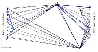
Figure 2 - Plan of the Control Network for the Latin inscriptions composed by five theodolite stations
