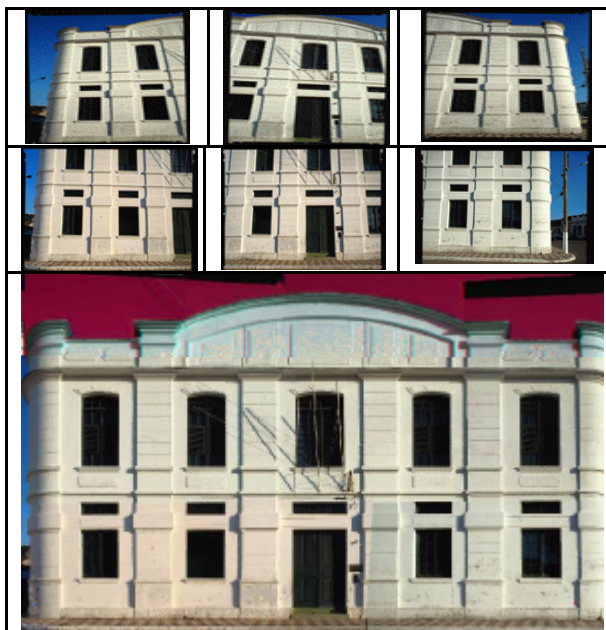
Figure 4 – Digital rectification of a facade from 6 sub-sets (original in colour)
