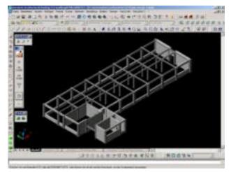
Figure 5b. 3D-model: Columns, beams, walls
