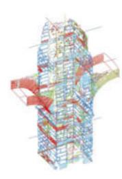
In the project of restoration of the aqueduct the criteria for the coding was primarily thematic based on aspects. As a result, to each building material used (granite, quartzite, ceramic, rubble concrete, metal...) corresponded a layer or group of layers. Some thematic layers gathered non-structural features such as paint stains, moss, lichen, oxide they served or to demarcate zones with different degrees of
