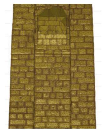
Fig. 3. Triangle mesh model of a pillar face.
