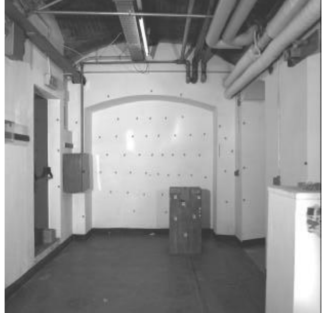
Figure 3. The Polygon Test where they are visible the target topographical finds by means of total station Leica TCRM1103
