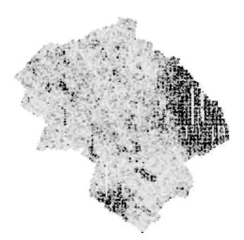
Figure 3. The DTM RMS values. The greyscale indicates the RMS values; higher values are darker and identify badly estimated DTM zones.
