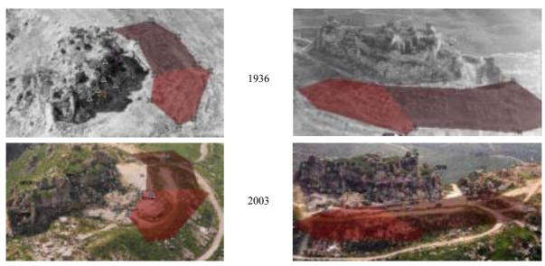
Figure 10. Archaeological structures are measured on the archive images of 1936 and the corresponding surface is shown on the photos of 2003
