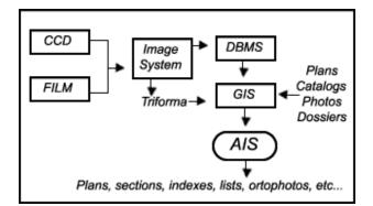
AIS system has two main cores: a digital photogrammetric system and the second core wich deal with the database management (the graphical one and the alphanummeric ones). This last core consists on a relational database gestor, a DBMS and a GIS software. The plattform chosen is Microsoft Windows NT.
