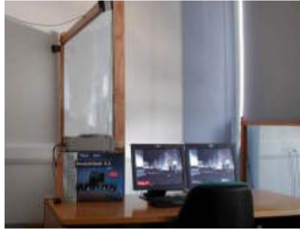
Figure 7. The visualisation set-up, showing the big screen and the mirror. The two monitors are used for control with each one giving a preview of what each eye will see on the big screen
