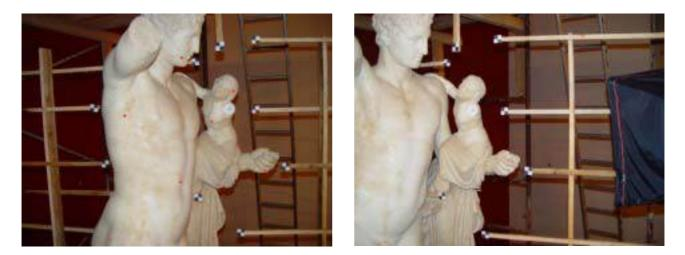
(a) left image (b) right image Figure 6. Stereopair of the upper part along the diagonal direction of the statue base
