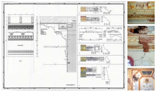
Figure 7a, 7b, 7c. The profiles of the three-dimensional projecting cornices of the interior walls in Room 101. These cornices were documented in 1:10, 1:5 and 1:2 scale. The photos show the severe damage on the cornices and the ceiling.
