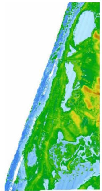
Figure 4: Color coded terrain model derived from laser scanner data.
