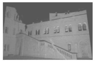
Figure 4: 3D Point cloud by IMAGER 5003
