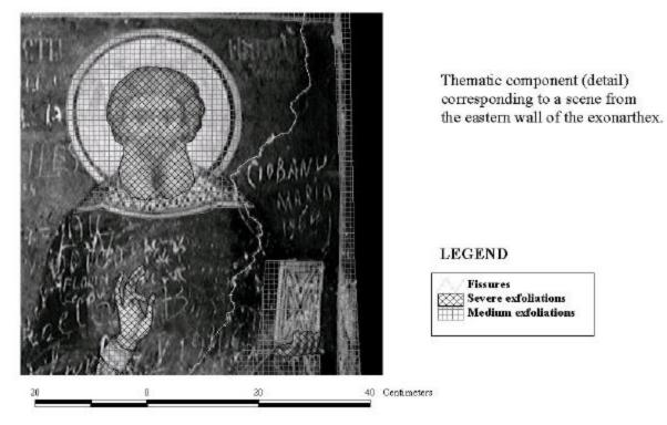
Figure 2. Thematic component overlayed to the graphic reference basis (detail)
