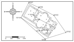
Figure 1. The polygonometric network.
