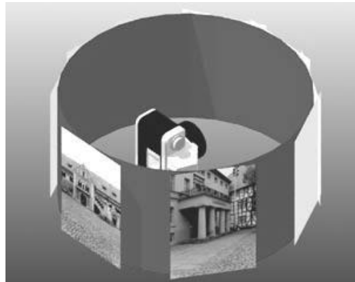
Figure 4: Principle of the segmented method for taking panoramic images
