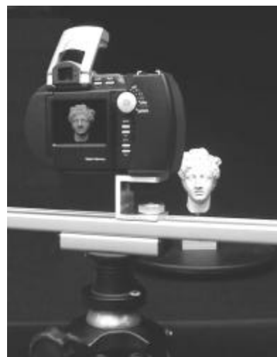
Figure 7: Rollei d7 metric assembled on a stereo bar recording a photo object.
