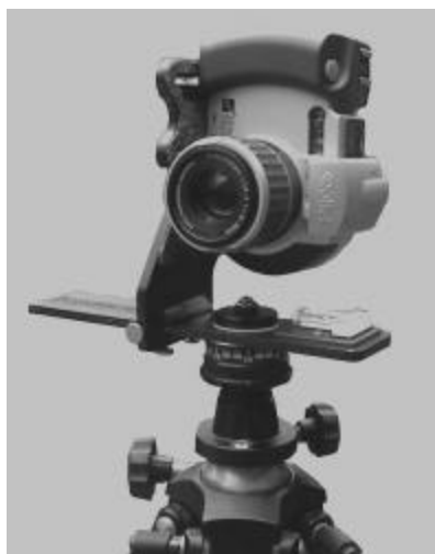
Figure 6: Rollei d7 metric fixed on a panoramic head for taking segmented 360 degree panoramas
