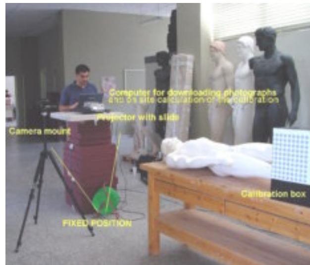
Figure 2. Set up of camera and projector during Kouros' plaster replica photography in ARF's lanoratory.
