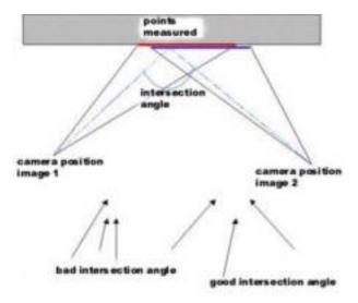
Figure 3. Principle of taking metric images
