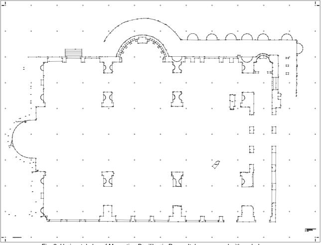
Fig. 2: Horizontal plan of Maxentius-Basilika, in Rome, Italy, measured with coded survey
