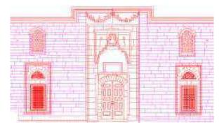
Figure 6. 3D vector plotting of Fatih Mosque northwest side
