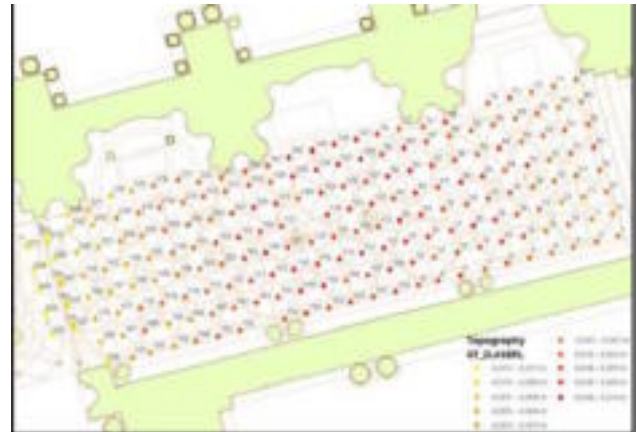
Figure 9. Comparison between the level height of the photogrammetric check points and the extracted height from the lattice (generated from the data laser scanner)
