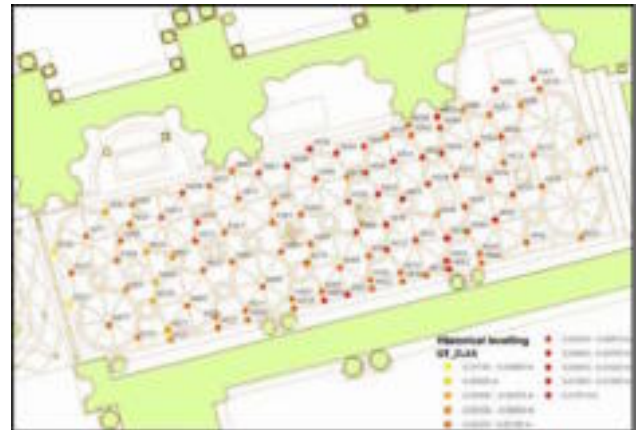
Figure 8. Comparison between the level height of the 2005 and extracted height from the data laser scanner (historical points)
