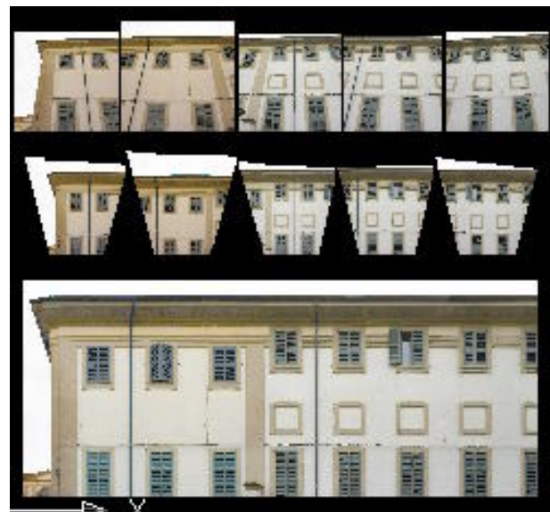
Figure 13. The taken, the corresponding rectified images and the mosaic realization. The images present for each front the rectified image, the horizontal and vertical profile, the dimensions of the tables, manageable with sw AutoCad, from a minimum of 30 MB for the smaller front to the maximum of 1,2 GB for the bigger fronts. For these ones, rectified images in different resolutions have been realized in order to help the files management
