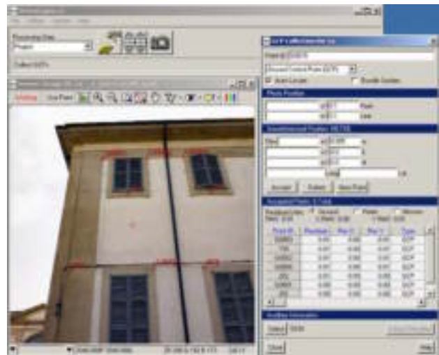
Figure 8. The procedure for the realization of a rectified image. The coincidence of the support points with the OrthoEngine software and the table showing the error residual in mm (maximum error 1 mm)
