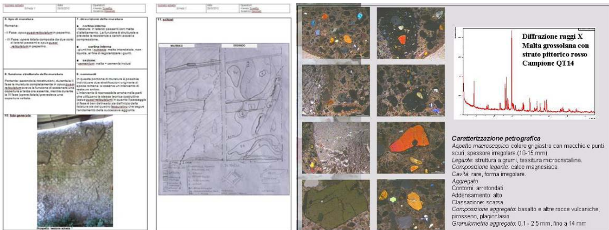
Figure 6. Example of compiled card with photos and sketches concerning the degradation of a plastered wall. Mineralogic and petrographic characterization of the mortar sampled from the opus caementicium wall.
