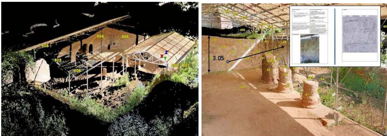
Figure 6. On the left: the textured point clouds; on the right an example how the materials data sheet can be linked to the 3D model.
