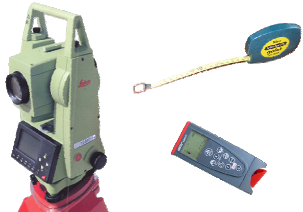
Fig. 2 – Total station (on the left), distancemetres (on the left-top) and rulers (on the left - below)
