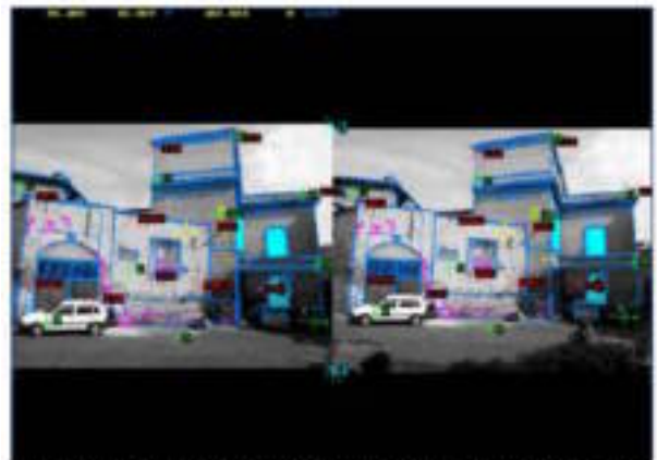
Fig. 10. Graphic interface of VSD. Stereopairs, control points and plotting are visualized
