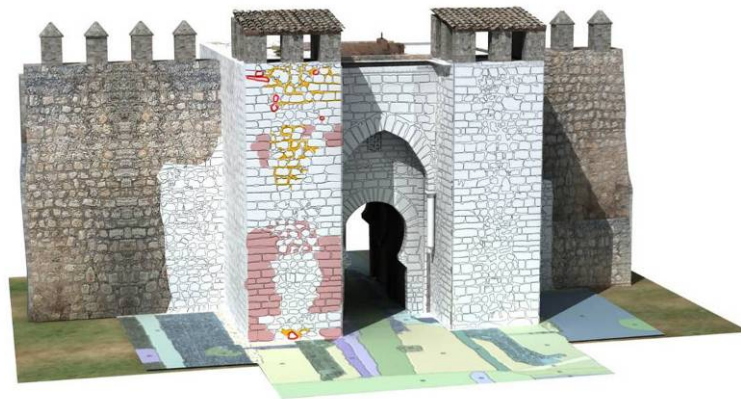
Figure 7. Integration and management of photogrammetric, archaeological and conservation data in the 3D reconstruction model of the Toledo Gate
