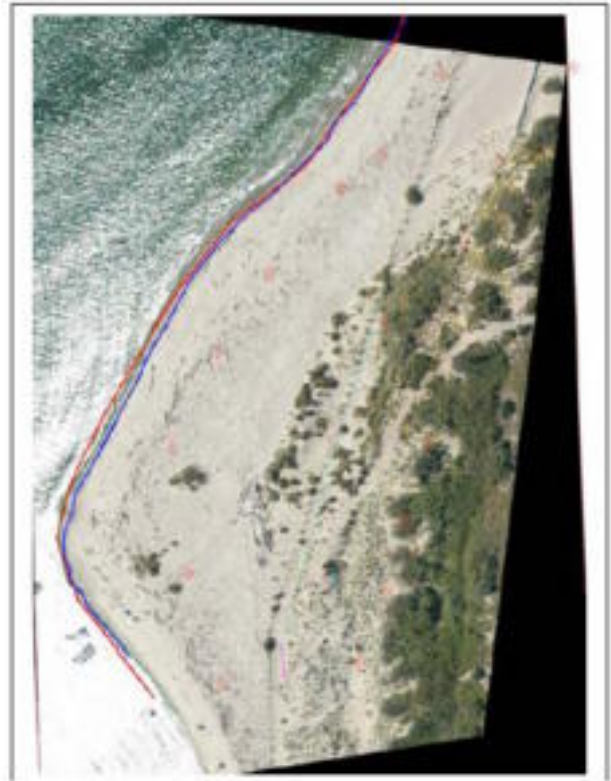
Fig. 8 Comparison of coastlines obtained with GPS (red), Stereorecording (blue) and rectification (green)
