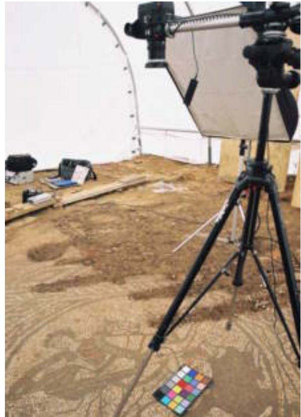
Figure 3. Camera and flash arrangement inside the tent
