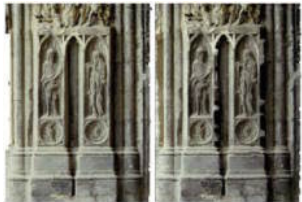
Figure 5. Example of an orthophoto from an edited stereomodel (left) and an unedited stereomodel (right).
