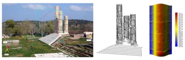
Figure 4: Examples of the Temple Columns, Linear Model and Column Surface Model
