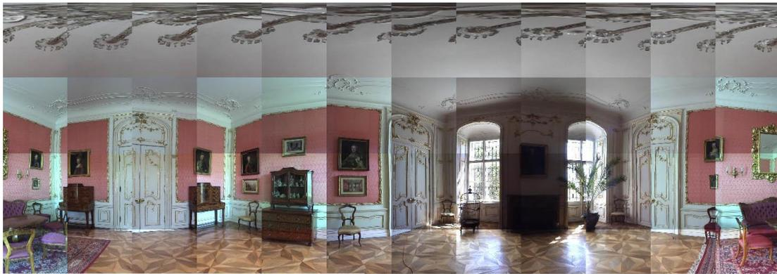
**Figure 8:** Results of laser scanning (distance image) and partial photos for point cloud rendering (Callidus CP3200)
