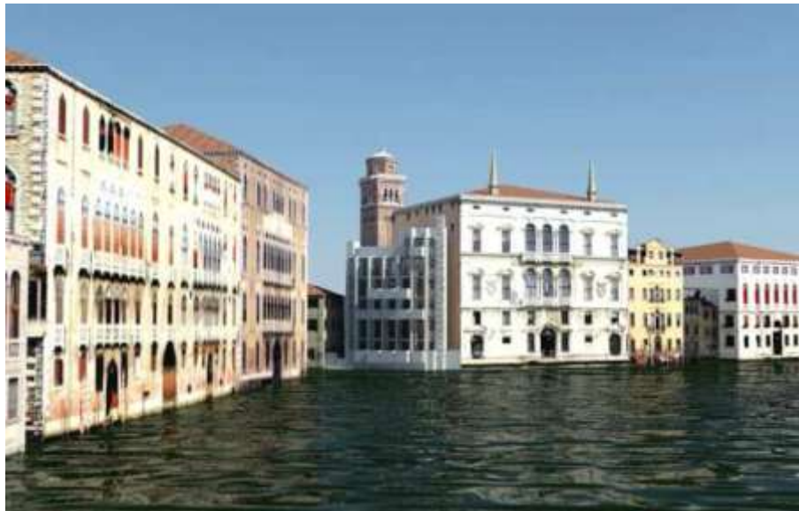
Figure 9: mock-up of the model in the 3d city model at the present day. Some mistakes are due to the use of simple volumes texturized by the orthorectified images of the facades.
