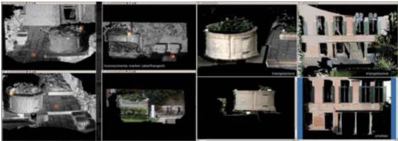
Figure 9. Details of the scans in Querini Stampalia garden. On right, triangulation and orthophoto from laser scanner survey
