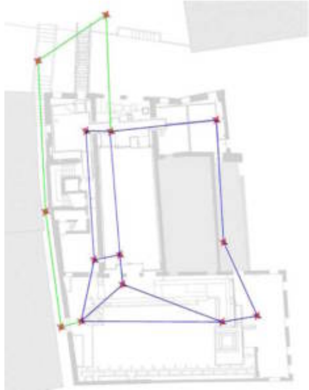
Figure 7. Scheme of topographic network
