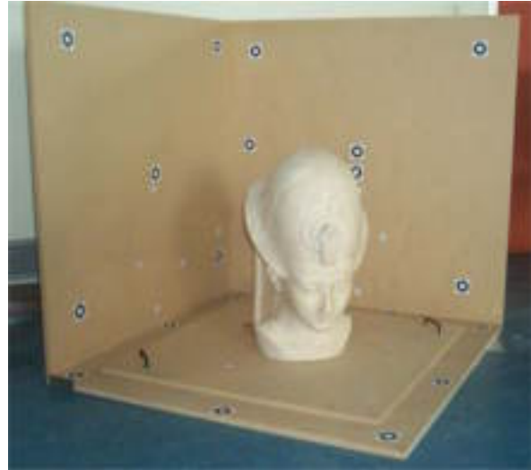
Figure 3 - Test scene for geometric measurements: a copy of Ramesse II bust kept in the Egyptian Museum in Turin
