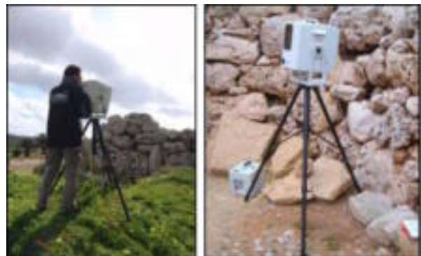
Figure 3. Leica HDS2500 laser scan
