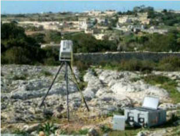
Figure 7. The Leica HDS 2500 laser scanner being used on site at Misrah Ghar il-Kbir, Malta.
