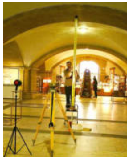
Figure . Crypt key stone monitoring with a modified 3 meters bar code levelling rod for the reading from the top.
