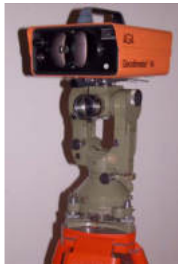
Figure 1: A distancemeter mounted onto the top of a theodolite
