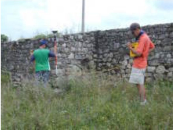
Figure 5. Kinematic GPS survey of the wall structures.
